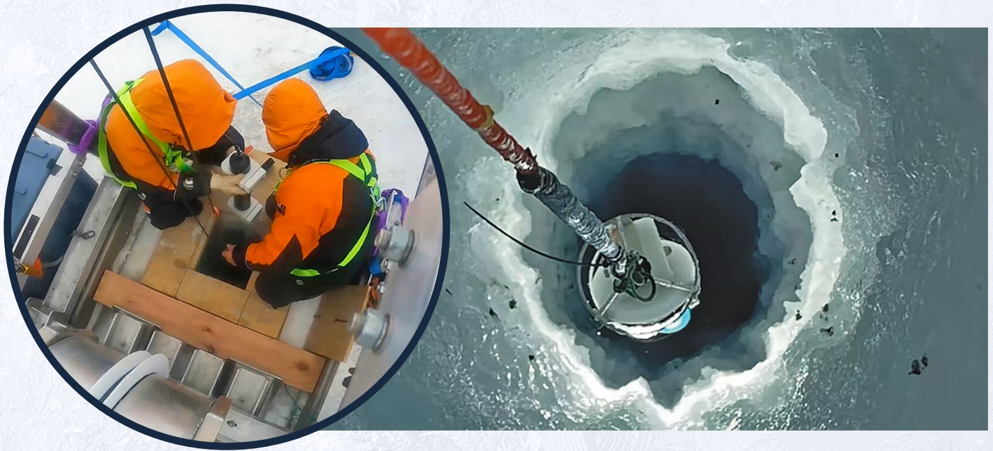
Scientists got their first glimpse into the hidden landscape in late 2021, when they drilled a borehole through 500 meters of ice and lowered instruments (inset) to observe the cavern below.
