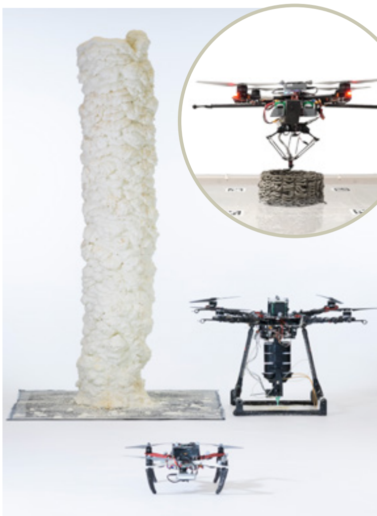
A larger BuilDrone and a smaller ScanDrone worked together to build a tower about 2 meters (6.5 feet) tall. A flying printer (inset) squirts out streams of a cement-like material.
